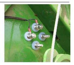
Keep in mind that the cable must be so long that the plug in the attached state is in the cab of the tractor. The excess cable length best to be fixed at a sheltered position at the press. The cable should not be reduced.
